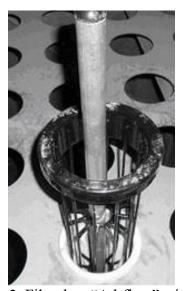
Pic. 2. Filter bag "Ad-flow" with the cage
