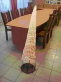
Pic. 8 Filter bag 3DESA filtrpatron for coal power station We are in procedure of discussion the next testing.
